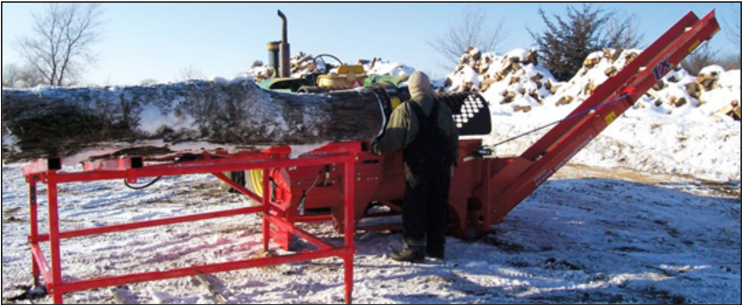
Red Salzbrun at the controls of his Wood Beaver 1x42 Green Speed firewood processor; deck at left holds logs in place, ready to feed into the processor.
