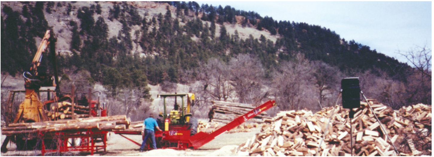
Resource Recovery Systems is the largest U.S. importer of firewood processors from Maaselan Kone Oy in Finland. The machines, powered by tractor PTO, are designed to be versatile, portable and economical.
