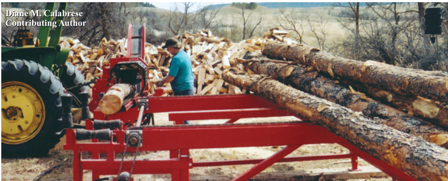
Walt Neiman cuts and splits ponderosa pine logs into firewood with a Wood Beaver 1X37 firewood processor; he also bought an optional two-strand live deck (shown) from Resource Recovery Systems.
